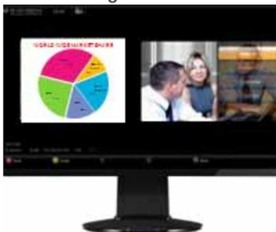
**Figure 8-3** depicts a PoP (Picture out Picture) view in which two images of different size are presented side by side.
