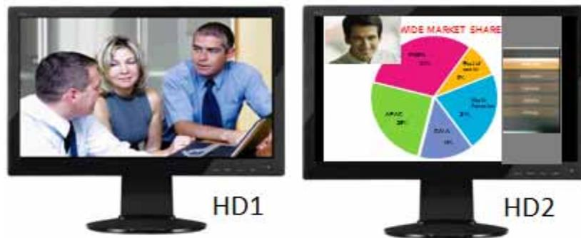
Seeing two images side by side and at the same size in one monitor is called PaP (Picture and Picture) view. See [Figure 8-2 on page 48](#) for a picture of the PaP view.
