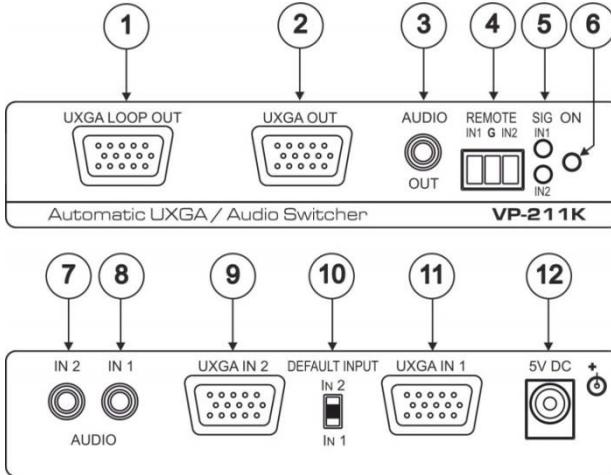
Figure 1: VP-211K Automatic UXGA / Audio Switcher
