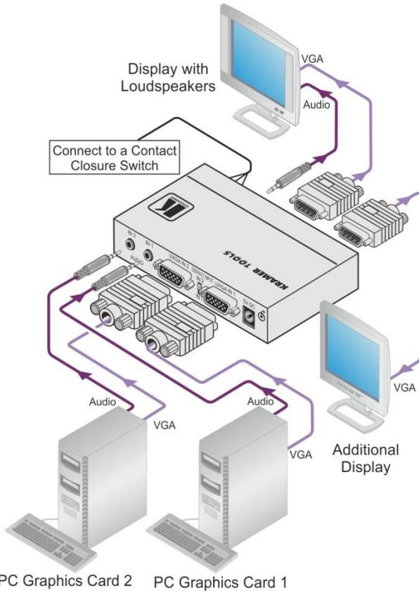
Figure 2: Connecting the VP-211K Automatic UXGA / Audio Switcher
